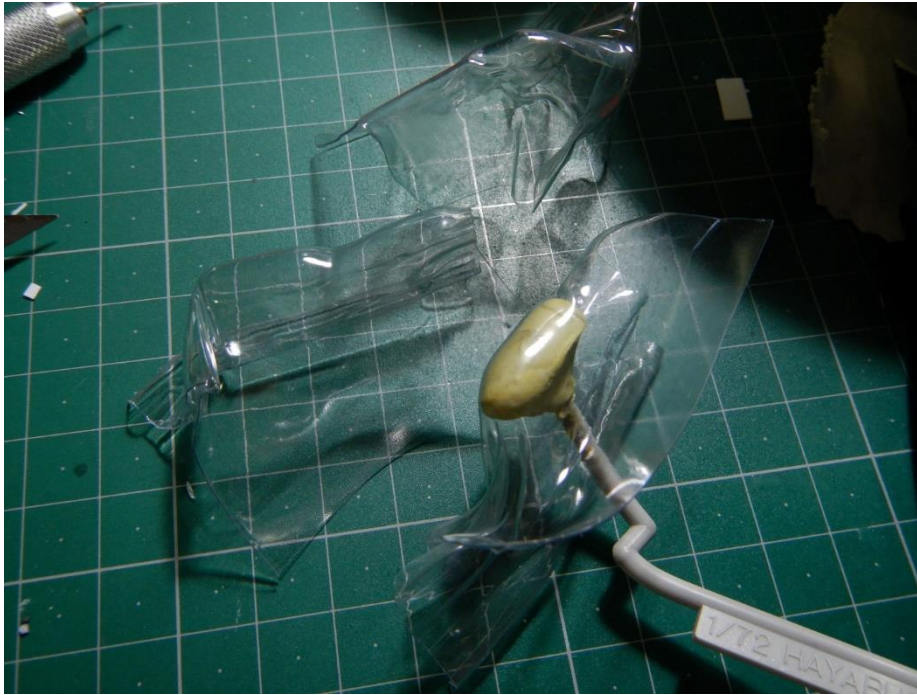
Figure 28. (31/12/2017) I wanted to present the canopy opened to reveal the cockpit rather than having it hidden behind a distorted canopy. This called for a vacuform replacement but I had still yet to build a vacuformer. After learning of crash-forming, I attempted to do this around the beginning of the build using a cut bottle, heating it over a BBQ grill at the time, and plunging it onto the original canopy. Unfortunately, this did not work well and the original canopy was distorted from the heat. After thinking and reading, my mistake was using polyethylene (Recycling code 1) which shrinks rather than melts when heated. I still hadn't given up on the technique and so salvaged the canopy and made a plug out of it by using original Milliput epoxy putty to reinforce and reshape it. A piece of sprue was also incorporated into the plug to hold it upright. After rummaging through my plant propagating equipment and remembering properties of weathered plastics among my containers, a spare PVC strawberry punnet (Recycling code 3) was found, cut and heated over a candle. This time things worked as expected and once soft, this was pulled over the plug quickly to form the shape and with great success too. Three copies were made and were ready for cutting.
