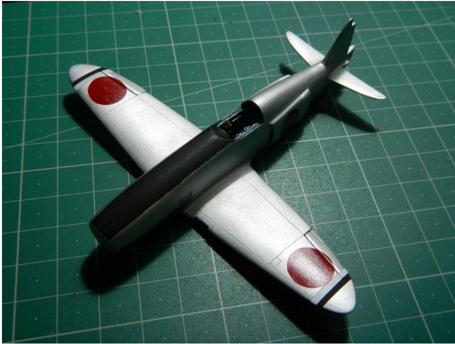
Figure 42. (10/01/2018) Painting is finally completed! The ailerons were first superglued into place before painting. Hinomaru were masked using Maketar's 1/72 Hinomaru masking set and airbrushed with Tamiya Red acrylic. Wheel wells, were airbrushed with my Aotake mixture. Engine exhaust panels were masked and airbrushed with Tamiya Gun Metal Acrylic. The front upper surface of the fuselage was airbrushed with Tamiya Flat Black. Finally, the distinguishing wing markings of the configuration of interest was masked and painted with Tamiya Flat White and Tamiya Flat Black. Next is the last stretch, attaching all completed pieces to the airframe.
