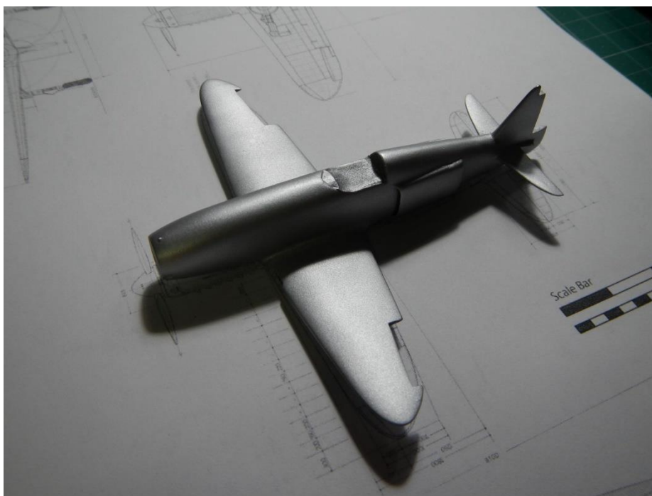
Figure 40. (09/01/2018) With the current heat wave starting to dissipate, progress resumed. The fuselage was primed with Alclad II Grey Primer, airbrushed with Tamiya Black, sealed with Pascoe's Long Life Floor Acrylic and finished with Tamiya Flat Aluminium. Next is the risky part, scribing panel lines through the paint. To help me with line positioning, a copy of Minoru Matsuba's blueprints was scaled down to 1/72 scale in Adobe Photoshop and printed for reference.
