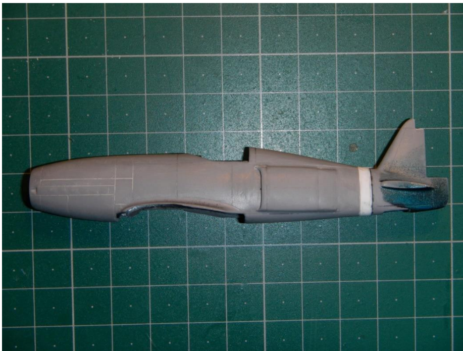
Figure 26. (29/12/2017) When measured properly, the entire fuselage including the propeller was short by 2.5 mm to scale. The fuselage was then extended by using 5 layers of cut 0.4 mm styrene strips and 2 layers of 0.25 mm styrene with the last being a closed bulkhead. This was then filed and sanded down to shape.
