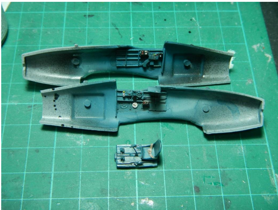
Figure 23. (26/12/2017) The cockpit interior was painted with a Hai-Ai-Iro mix based on the recommendations Aviation of Japan's recommendations in their Ki-78 kit blog post ( http://www.aviationofjapan.com/2014/12/some-observations-about-ki-78.html ). This mixture was made with a 1:1 ratio Tamiya Light Grey and Tamiya Royal Blue acrylics. Smaller details were hand painted before applying a matte brown wash over it, lazily made with a very thin mix of Tamiya Red, Yellow and Flat Black acrylics. All non-metallic acrylics up to this point were thinned with my homebrewed acrylic thinner.
