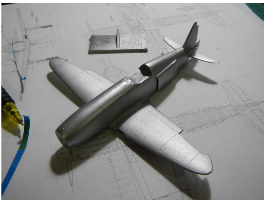
Figure 41. (10/01/2018) After around 3 hours, scribing has been completed. Although it was very risky, this method is not as difficult as you'd think and is probably by far the most rewarding for the finest and most realistic lines in this scale even though it is still not accurate (technically, almost no panel lines should even be present in 1/72 scale). This was my first attempt at using this method on an entire model and of course there were mistakes along the way. However, in the case of Flat
